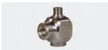
3/8" IG : 3/8" AG. DN 10. Max. 30 U/min / 90 °C
